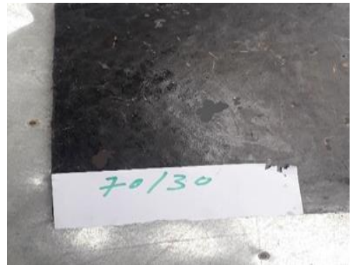
Fig 3d. Sample created with a composition of 70% human hair and 30% resin and filler
